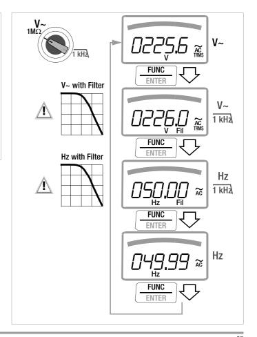
5.1.3 Alternating Voltage and Frequency Measurement V AC and Hz with Selectable Low-Pass Filter (METRAHIT AM X-TRA / AM TECH / AM PRO / OUTDOOR / SECULIFE HITAM/MD only)
